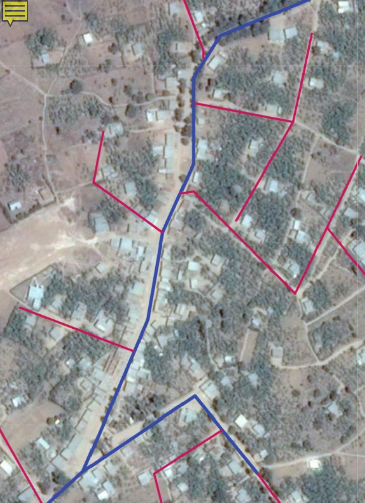
Example micro-grid topology Blue = 240V AC line Red = 48V DC line
