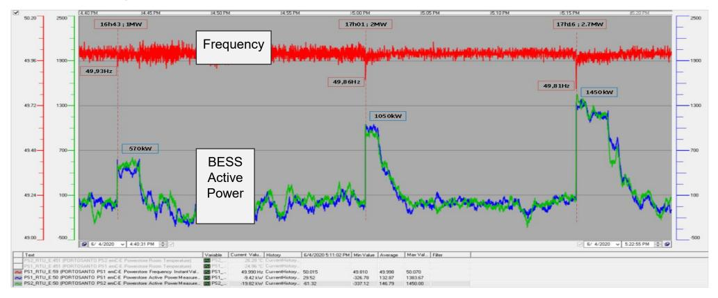
BESS response during DG trips, sustained the frequency within a safe margin and avoided load shedding.
