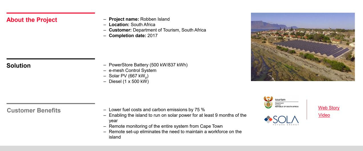
Grid Edge Solution enables Robben Island to run on solar power for at least 9 months in a year
